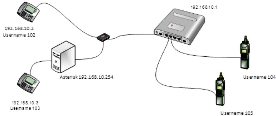
Figure 1 Example showing radios, phones and an Asterisk SIP proxy connected through BASICS Radio Relay
